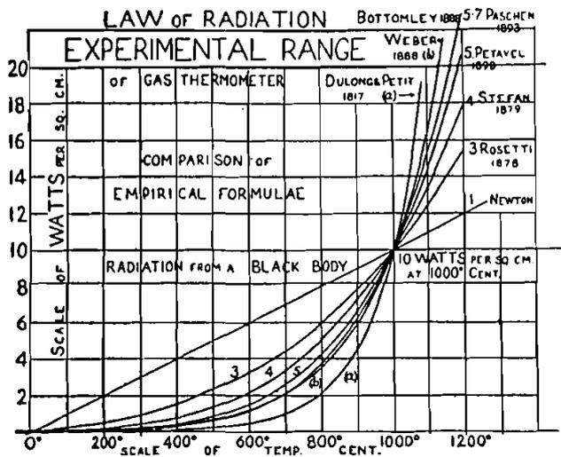
Figure 9 Formulas for radiation, experimental range [35].
